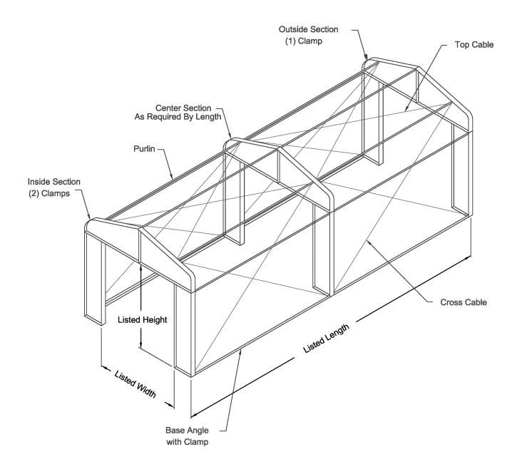
Frames are shipped complete with all assembly hardware including diagonal cables. (Anchors Not Included)
